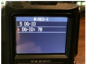
To set Wires-X DG-ID on a FT2DR: Press DISP button for 2 seconds Press Wires-X soft button briefly Turn DIAL to select 5. DG-ID Press 5. DG-ID Turn DIAL to select 70 Press BACK button three (3) times YAESU ARCOU YAESD YAESU 2, 50 .... 2, 50 ..... 17:13 17:13 SETUP MENU SETUP MENU WIRES-X
