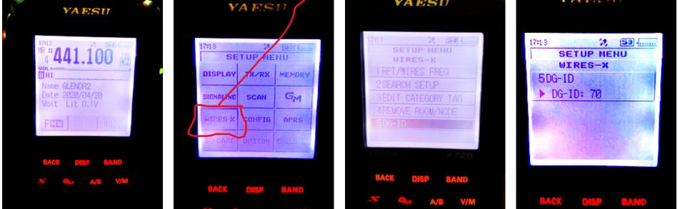
To set Wires-X DG-ID on a FTM-400: Press DISP button for 2 seconds Press Wires-X soft button briefly Turn and press DIAL to select DG-ID TX Turn DIAL to select 70 Press DIAL to save change Press BACK button two (2) times
