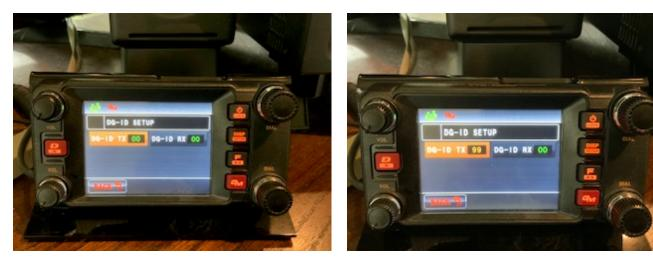
To set Wires-X DG-ID on a FTM100D: Long press DISP Turn DIAL to Wires-X #7 Short press DISP Turn dial to DG-ID #2 Short press DISP Press Back button twice
