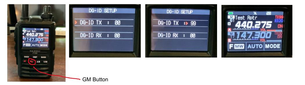
To set TX DG-ID on a FT2DR: Press GM button for 2 seconds Press GM button briefly Turn DIAL to set desired TX DG-ID Press BACK button twice
